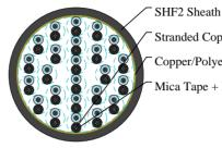
SHF2 Sneath Stranded Copper Conductor Copper/Polyester Tape + Drain Wire Mica Tape + HFEPR Insulation
